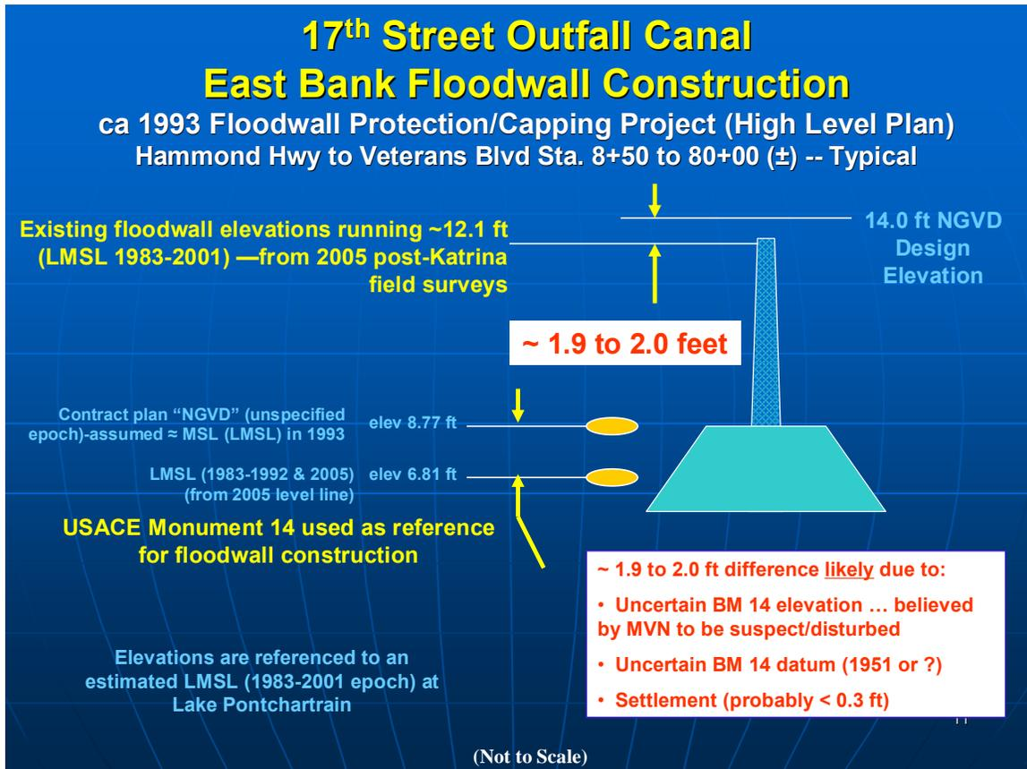
Figure 47. Design versus current floodwall elevation—East Bank 17th St. Outfall Canal.
