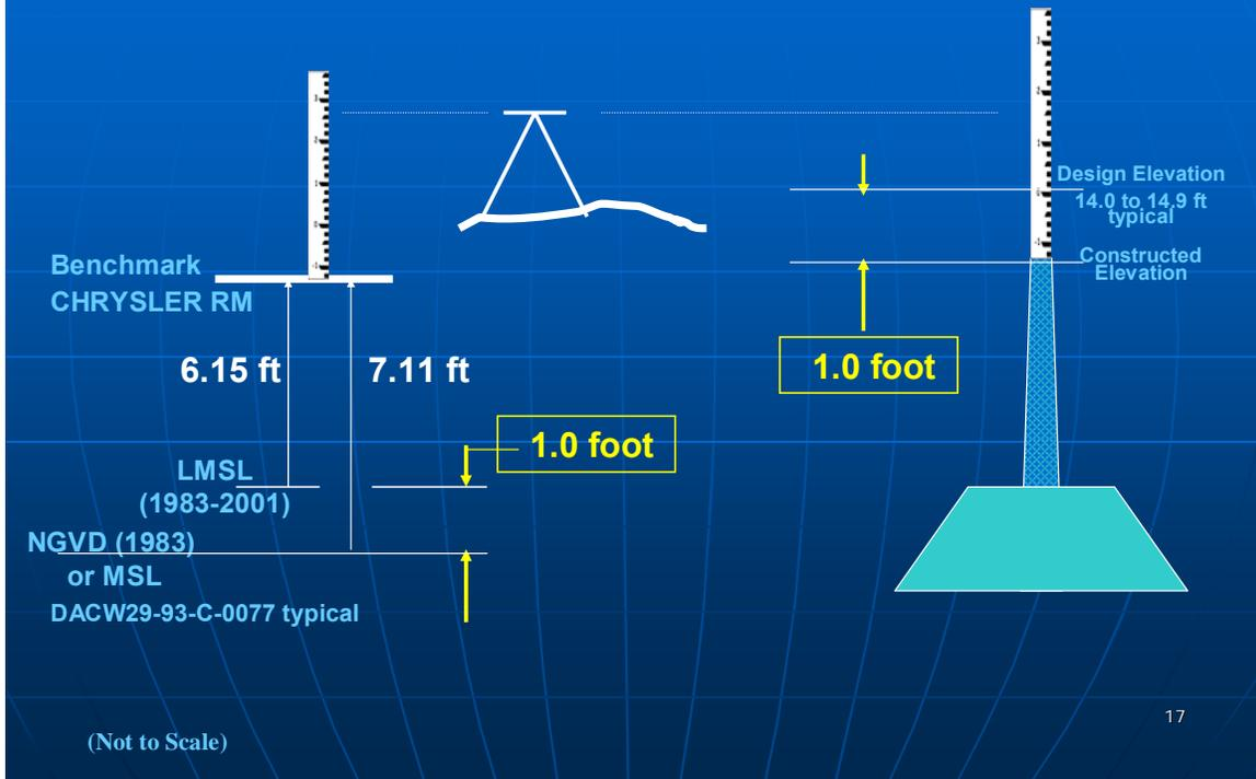
Figure 37. Impact of using NGVD elevation instead of LMSL elevation for construction stakeout of Orleans Avenue Outfall Canal floodwall construction (DACW29-93-C-0077). (Elevation differences are rounded to the nearest tenth of a foot.)
