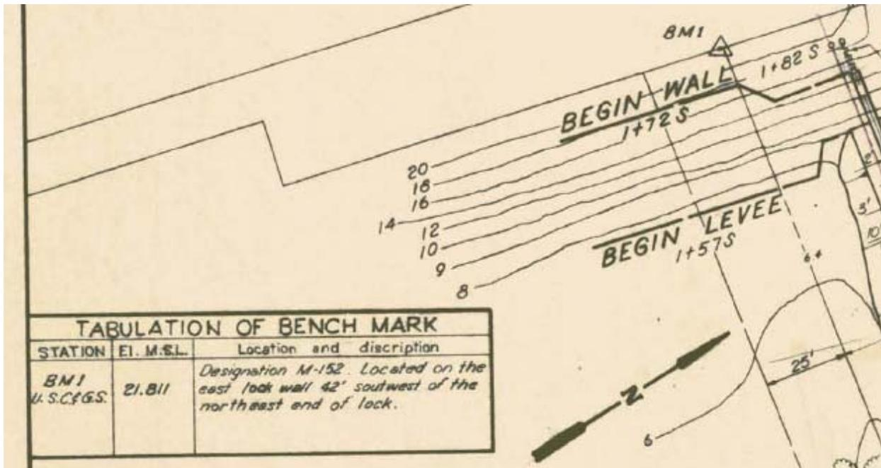
Figure 48. Location and description for Benchmark BM 1 (M 152 USC&GS) at IHNC Lock.
