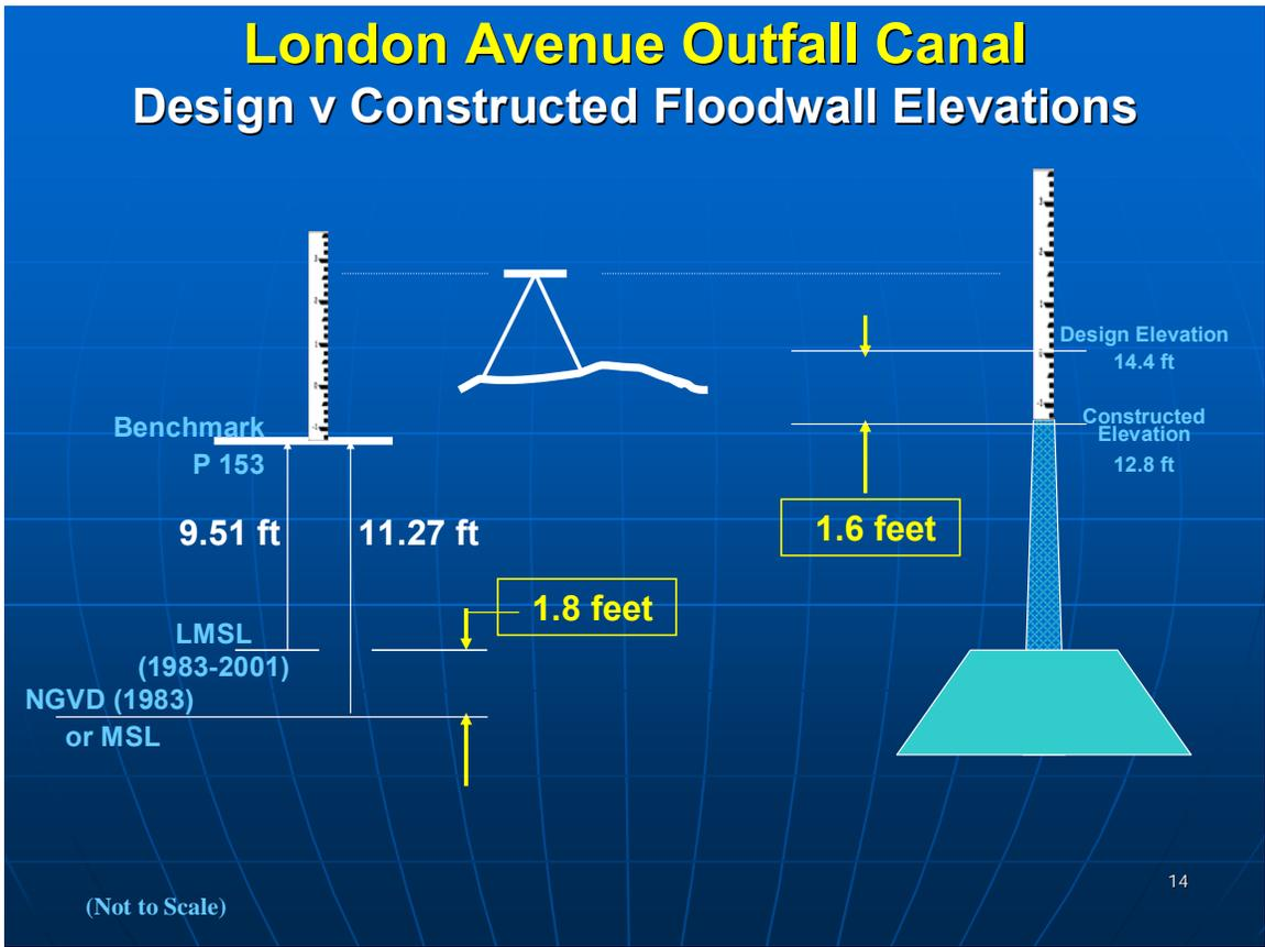
Figure 42. Impact of using NGVD elevation instead of LMSL elevation for construction stakeout of London Ave. Outfall Canal floodwall construction.
