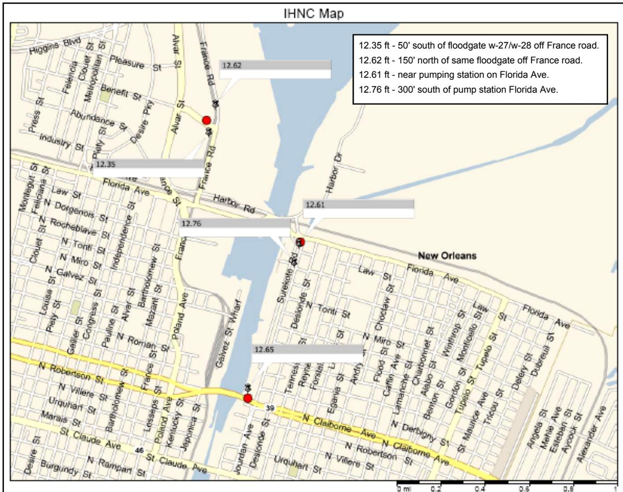
Figure 51. Selected post-Katrina elevations on IHNC Floodwalls.
