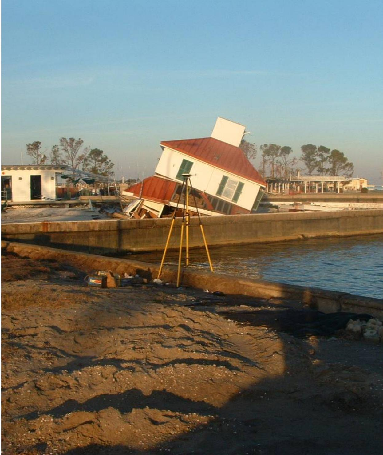
Figure 34. IPET GPS surveys in December 2005 at Benchmark ALCO on seawall bulkhead at USCG station vicinity NOAA New Canal Gauge (3001, Inc.).
