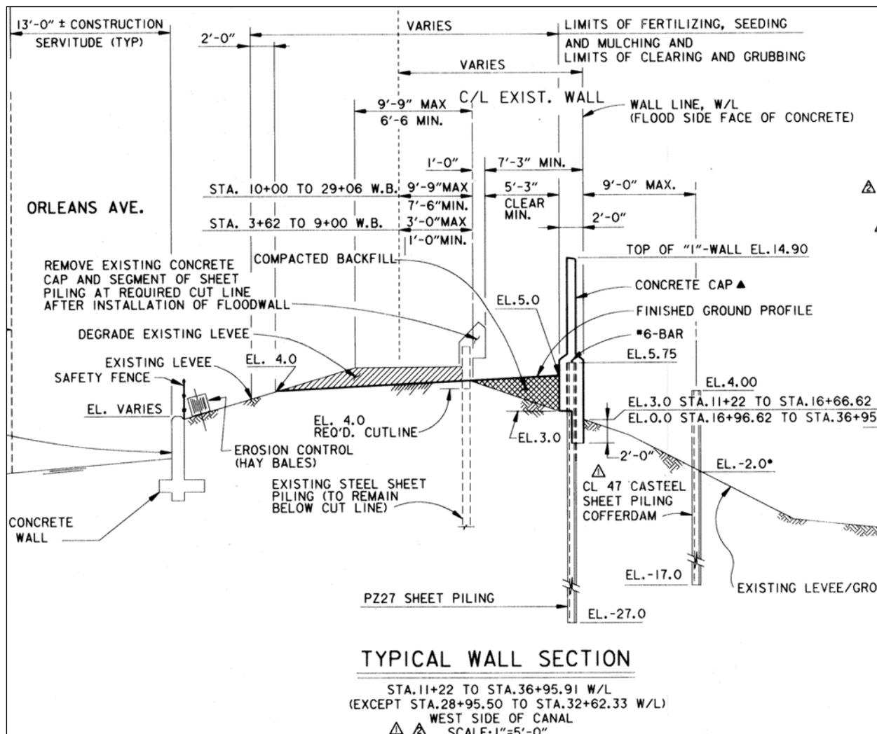
Figure 35. Typical I-wall section at elevation 14.90 ft (DACW29-93-C-0077).
