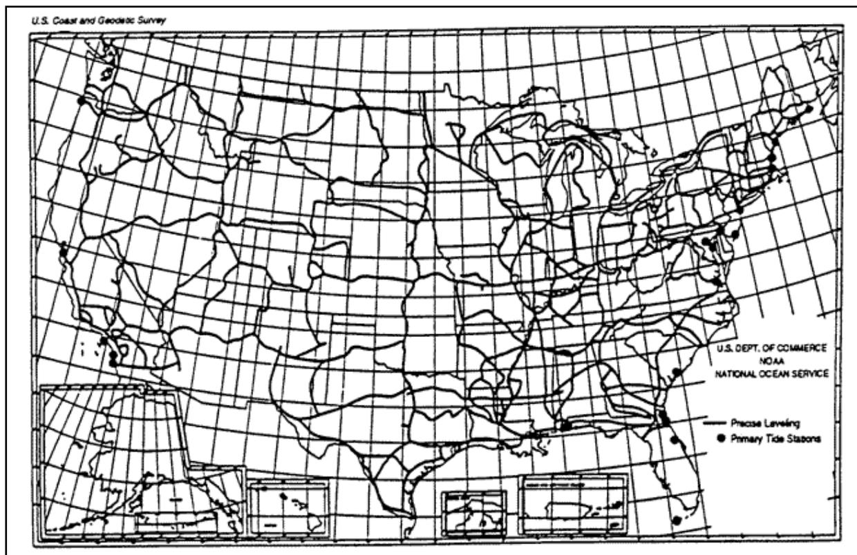
Figure 1. Precise level lines and tide gauges used to define the NGVD29 datum.
