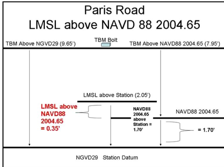
Figure 21. Methodology for determining LMSL (2001-2005 NTDE) – NAVD88 (2004.65) relationship at USACE water level stations.
