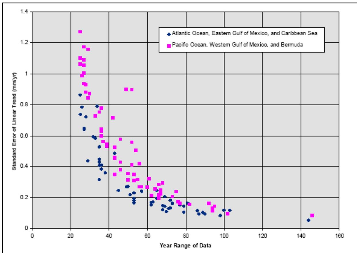
Figure 26. Standard error of linear LMSL trends versus year range in data.
