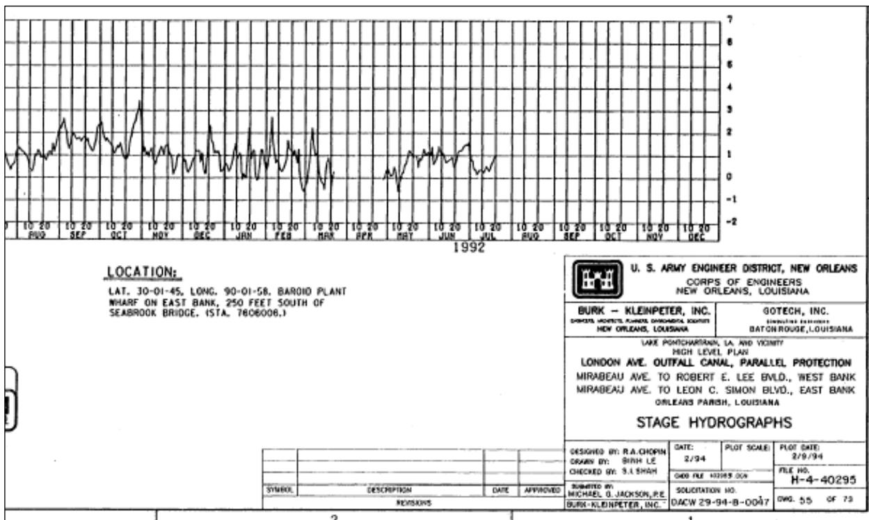
Figure 40. Typical portion of stage hydrograph on London Avenue Canal depicting 1+ ft superelevation based on the gauge at the Seabrook Bridge in the IHNC (DACW29-94-C-0079 (94-B-0047)).
