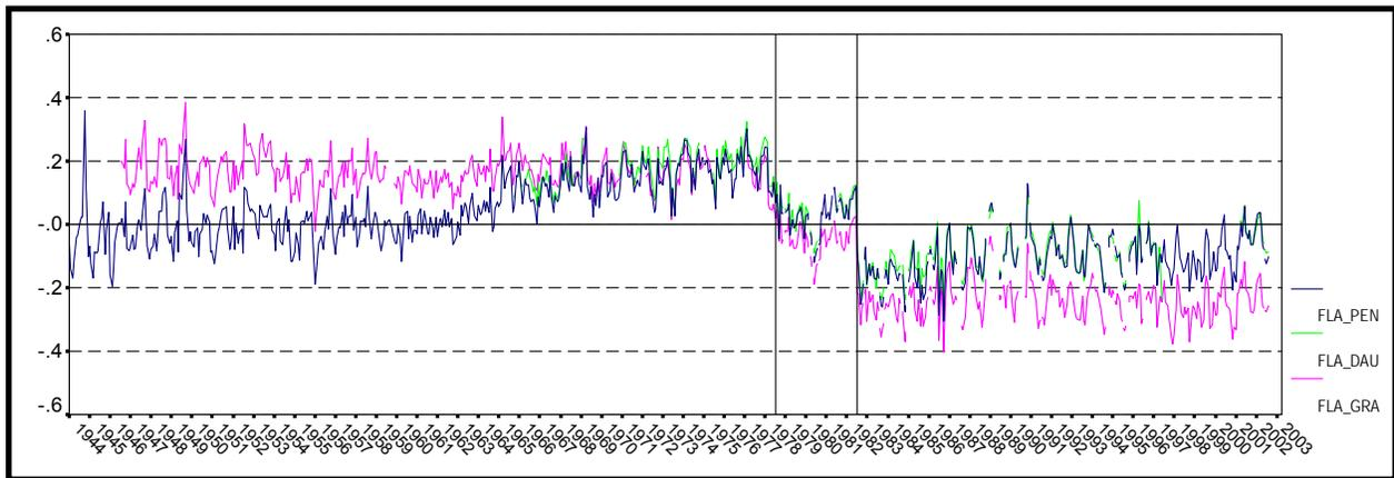
Figure 31. Three separate time series derived from simultaneous comparison of USACE Florida Avenue data with NOS data identifying significant datum shifts near 1978 and 1982.
