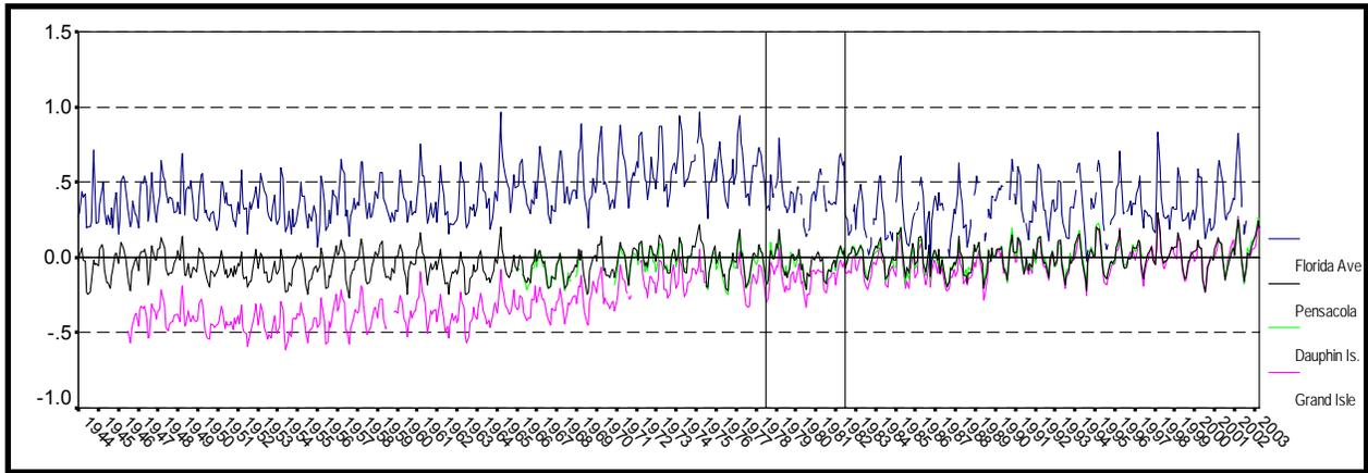
Figure 30. Possible datum shifts identified from raw USACE data through comparison with NOS data series at Pensacola, Dauphin Island, and Grand Isle.
